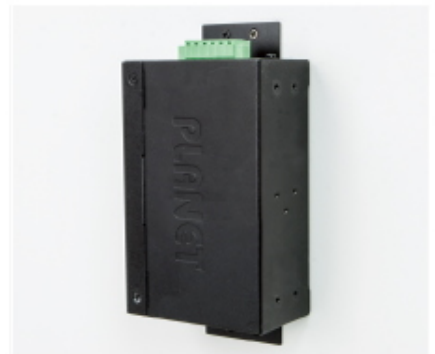
Side Wall Mounting (Space saving)
